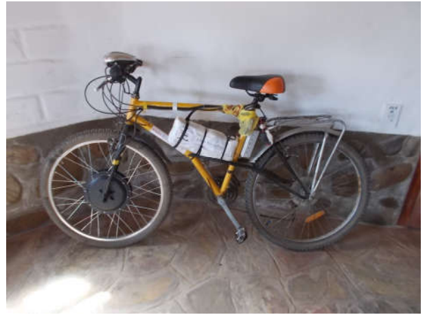
Advanced prototype; 350 W front wheel motor, 15 Ah Li battery
