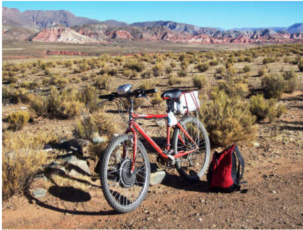
First prototype; 350 W front wheel motor, 15 Ah Pb battery
