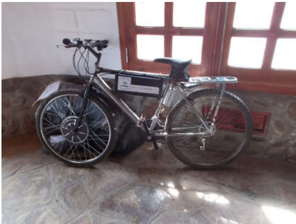
Advanced prototype; 500 W front wheel motor, 20 Ah Li battery
